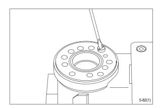
(22) Grease the O-ring with mineral oil approx. viscosity 500 cSt at 20°C.
