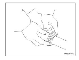
(2) Install the rod seal to the position in the gland applying a slight coat with grease prior to install.
