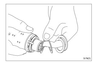
(11) Press out the cross pin. Use the special screw from the end cover.
