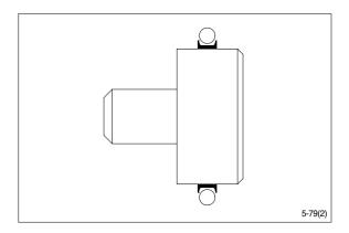
(12) Hold the outer part of the assembly tool in the bottom of the steering unit housing and guide the inner part of the tool right to the bottom.
