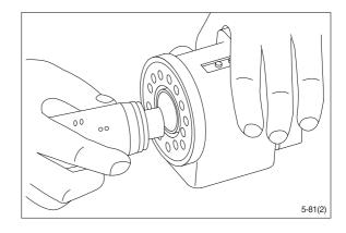
(19) The spool set will push out the assembly tool guide.
