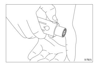
(14) Remove dust seal and O-ring.
