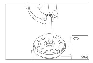
(25) Place the cardan shaft as shown - so that it is held in position by the mounting fork.
