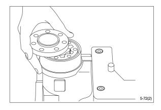
(3) Lift the gearwheel set(With spacer if fitted) off the unit.
