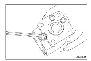
(17) Shake out spring and piston. The valve seat is bonded into the housing and cannot be removed.
