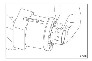
(10) Take ring, bearing races and thrust bearing from sleeve and spool. The outer (Thin) bearing race can sometimes "stick" in the housing, therefore check that it has come out.
