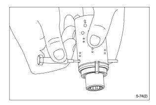
\*\* A small mark has been made with a pumice stone on both spool and sleeve close to one of the slots for the neutral position springs(See drawing).
