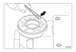
(21) Screw the threaded bush lightly into the check valve bore. The top of the bush must lie just below the surface of the housing.
