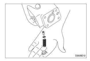
(18) The pressure relief valve is now disassembled.
