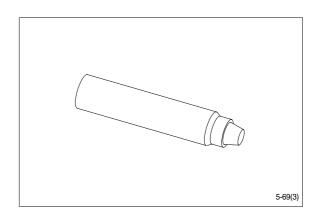
(4) Assembly tool for cardan shaft.
