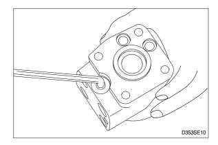
(16) Unscrew the setting screw using an 8mm hexagon socket spanner.
